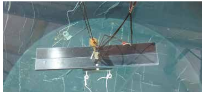
VLF Transducer with cantilevered bender design. High power, very Low frequency, full ocean depth transducer designed to operate in the 10Hz to 1000Hz range.
