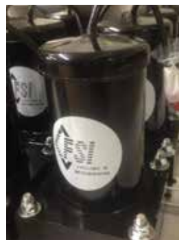
A high power 1-10KHz tonpilz
