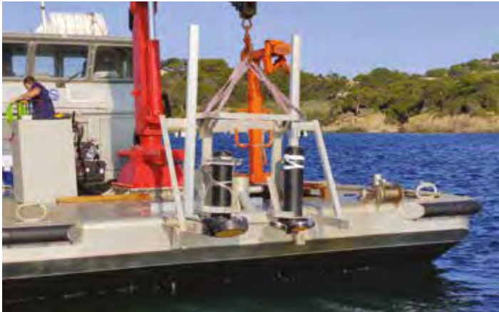
Figure 3: Signature100 and Signature55 in aluminum frame in standing position to prevent losses due to drag (left) and in deployed position as viewed from above (right).
