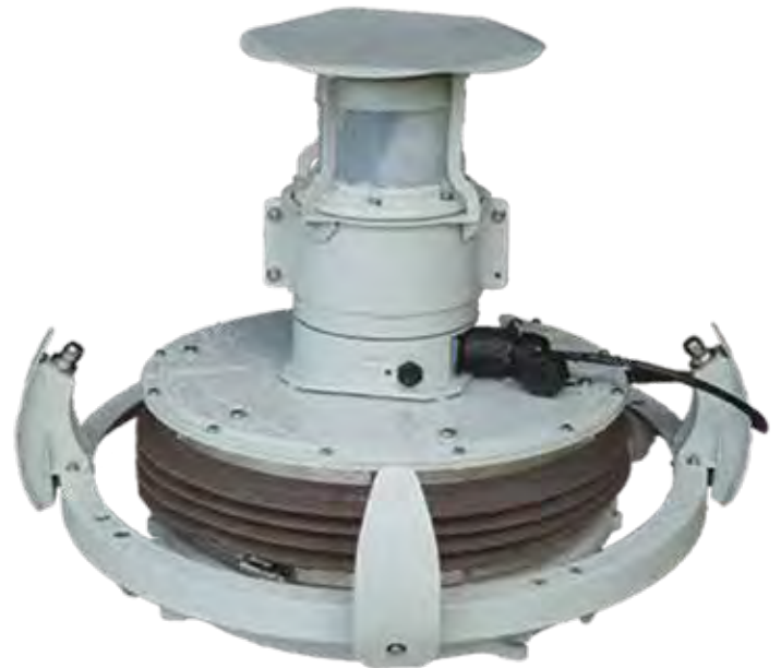
Figure 1: 360° camera installed on RSM
