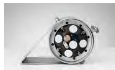
Vessel-mounted current profiler
