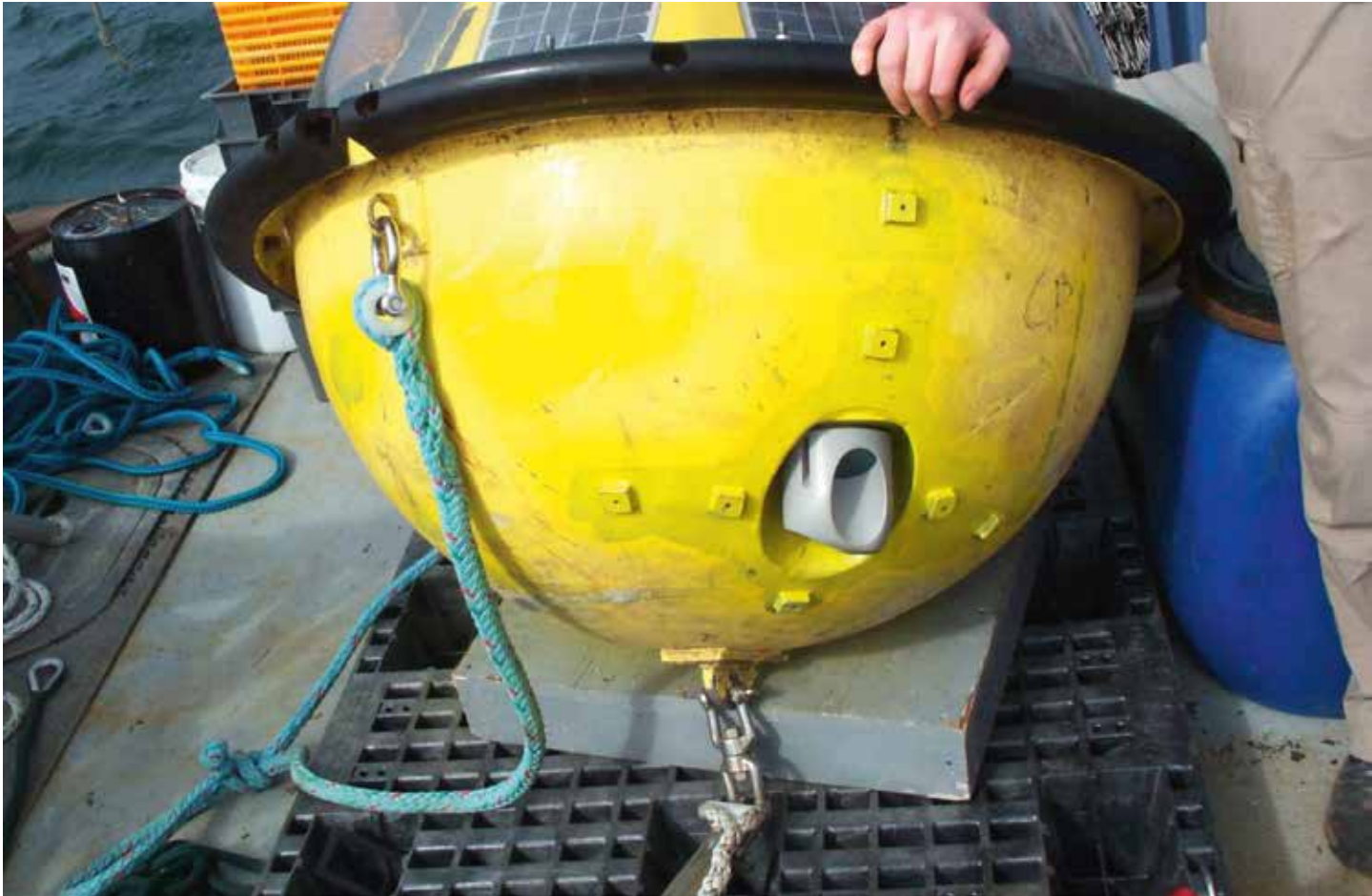
A Nortek Aquadopp Profiler mounted in a TRIAXYS™ with Currents Buoy
