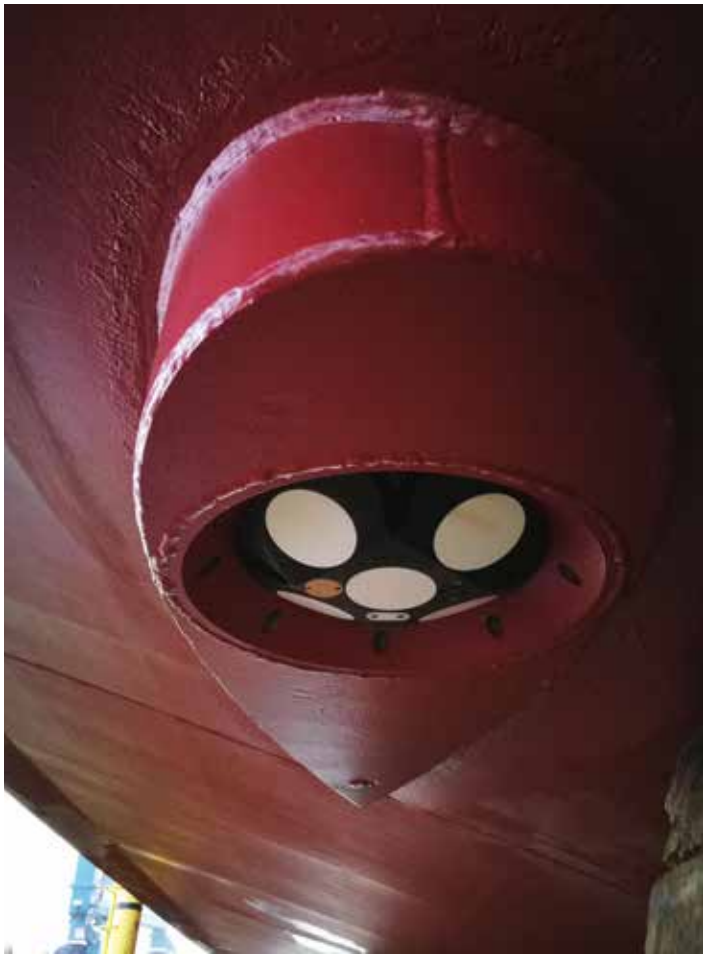
The Nortek Signature500 VM, hull-mounted on the vessel Geo Focus
