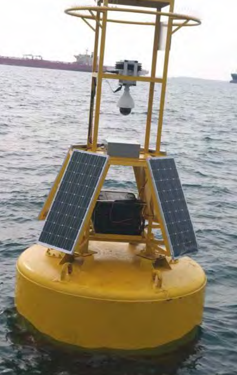
Figure 4: RSM 400 with PTZ camera installed on a buoy
