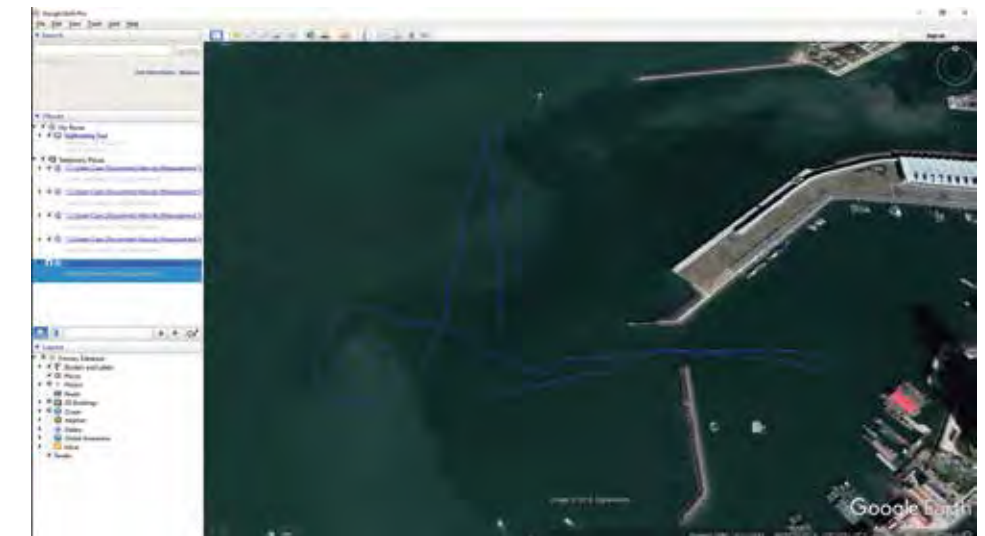
Exported data (in .kml format) showing the tracks sailed in Google Earth. The crew carried out so-called "lines" of current surveying inside and outside of the harbor to identify the differences in the currents' velocity and direction in these two locations.
