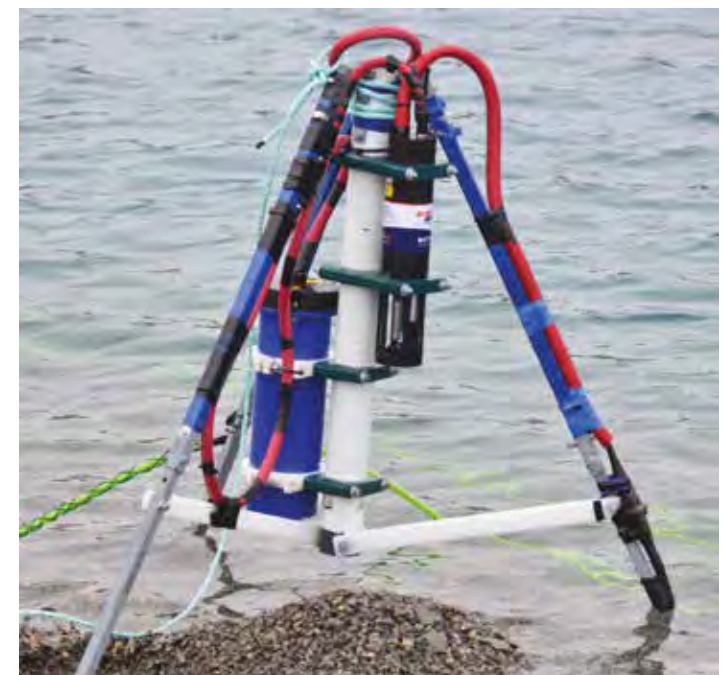
Figure 4 - Metrec•X multiparameter sonde with UV biofouling control ready for 12-18 month deployment (Image courtesy of Ocean Networks Canada)
