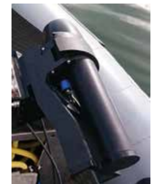
Fig. 3. The 3D 200kHz sonar integrated with Applanix Wavemaster for pole installation.
