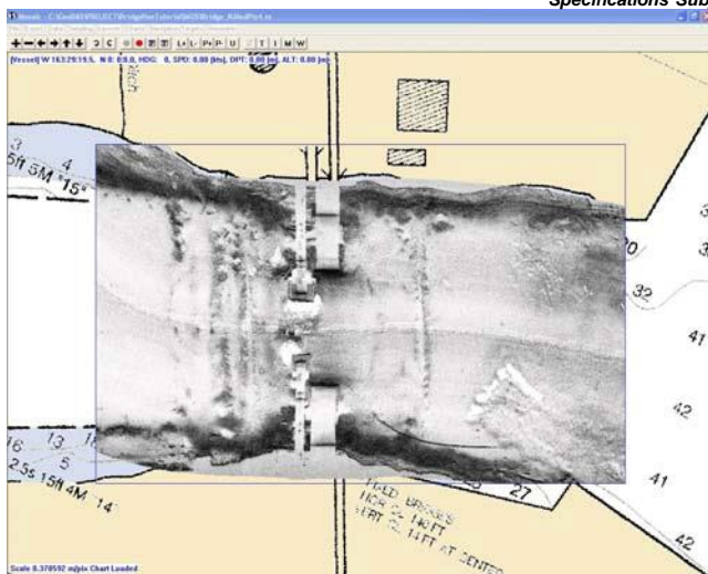
HMS-1400 sidescan image indicating bridge scour
